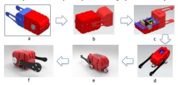
Fig. 1. Three iterations design of new module. a-c the first interations, d-e the second interations, f the last one.
