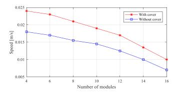
Fig. 8 Swimming speed variation with respect to the number of modules.
