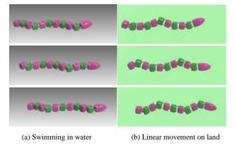
Fig. 7 Snapshots of amphibious locomotion with 11 modules eployed with covers, using control parameters A=45.0, T=1.0,  $\varphi$ =2.1 and O = 0.0.
