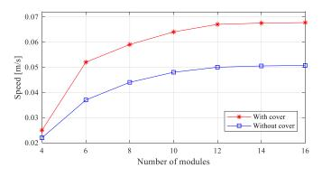
Fig. 9 Speed variation of linear movement on land with respect to the number of modules.
