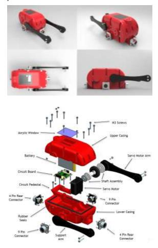
Fig. 2. Improved modular robot design
