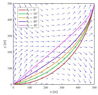
Fig. 5 The variation of ship trajectories with respect to different initial orientations.
