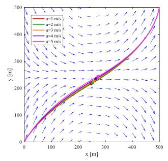
Fig. 6 The variation of ship trajectories with respect to different ship speeds over ground.
